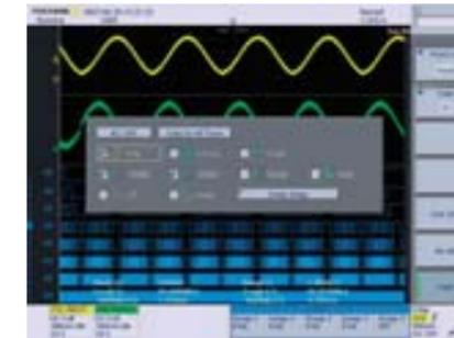
Time domain waveform parameters such as pulse width, interval, and delay can be measured automatically for logic signals as well.
