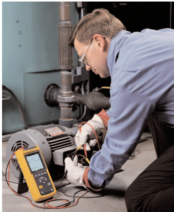
Using the Fluke 43B Power Quality Analyzer for average watt measurements.
