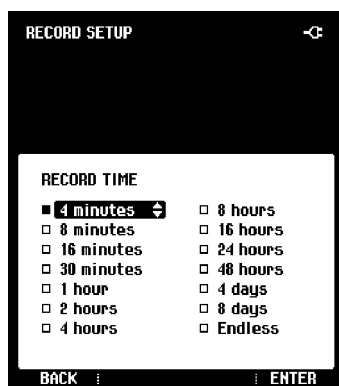
Fluke 43B recording mode with record time selections from four min to endless (16 days).
