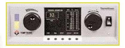
Model TP04100A ThermoStream® System, compact in size for benchtop use, provides precise, temperature controlled air from -20° to +225°C for thermally testing, cycling and characterizing components, hybrids and modules at the tester site or on a printed circuit board.
