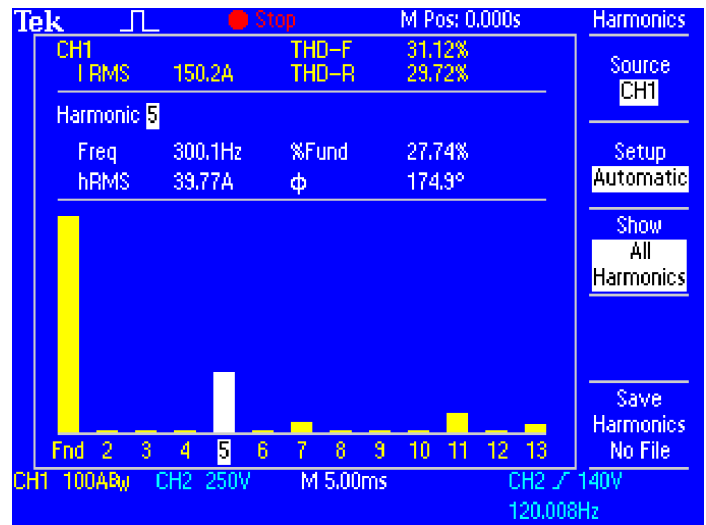
Conduct harmonic distortion measurements with TPS2PWR1 software.
