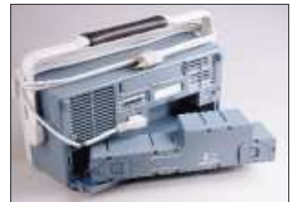
TDS 3BAT – Battery Pack being installed.
