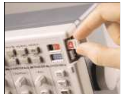
Application Module being installed.
