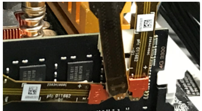
P77STFLXB solder down, flex-circuit accessory provides a probing solution for DDR4 and LPDDR4 electrical validation when used with Nexus XH Series Interposers.
