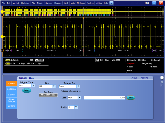
Triggering on a specific data value on the MIL-STD-1553 bus.
