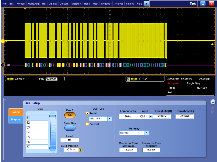
MIL-1553 bus setup, showing dual threshold settings.
