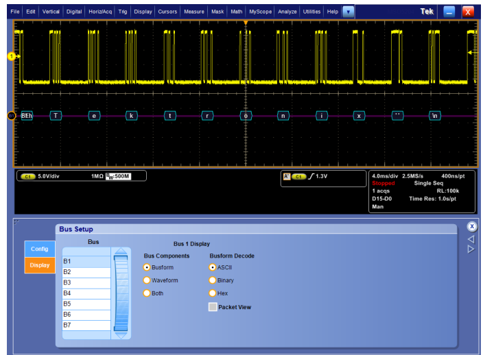
Color-coded RS-232 bus display, showing ASCII display format.
