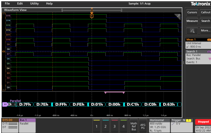
Digital channel trigger and decode
