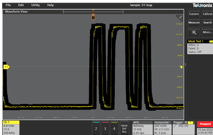
Limit mask test based on golden reference signal
