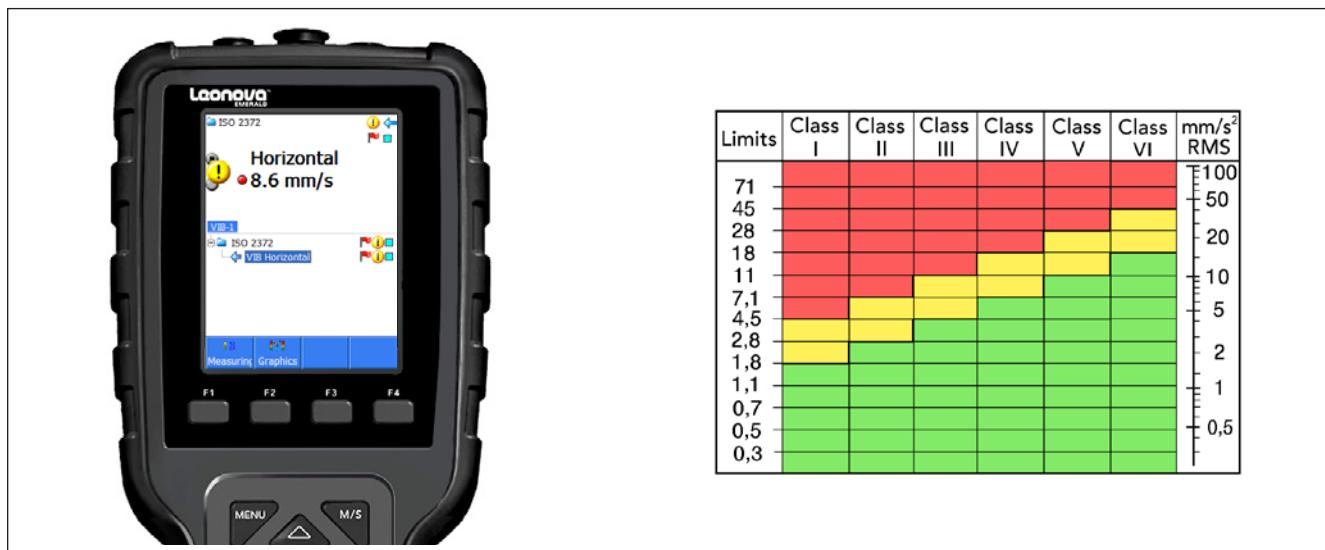
Broadband vibration measurement is the most widely used and cost-efficient method for the diagnosis of general machine condition. There are two ISO recommendations concerning this type of machine condition monitoring; the much used ISO 2372 and the more recent ISO 10816, which is a ongoing replacement of the older standard.
