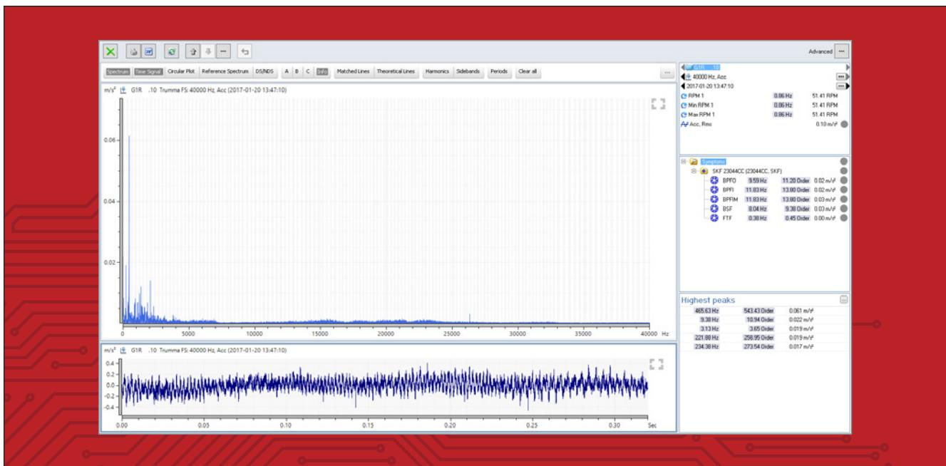
Rule-Based Evaluation (RBE) is a module in Condmaster Ruby. The purpose of RBE is to give the user guidance on what to do when certain alarm conditions are met. RBE is an excellent tool in Product Integrated Maintenance (PIM).
