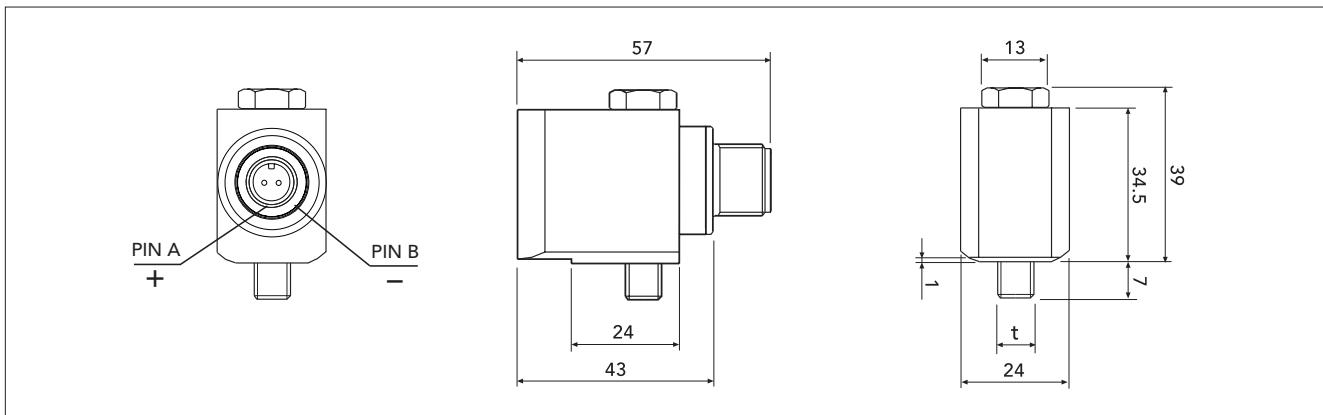
The vibration transducer SLD144S is a piezo-electric accelerometer of compression type with side entry and built-in electronics, designed for vibration monitoring of industrial machinery. The electrical signal is isolated from the transducer housing.
