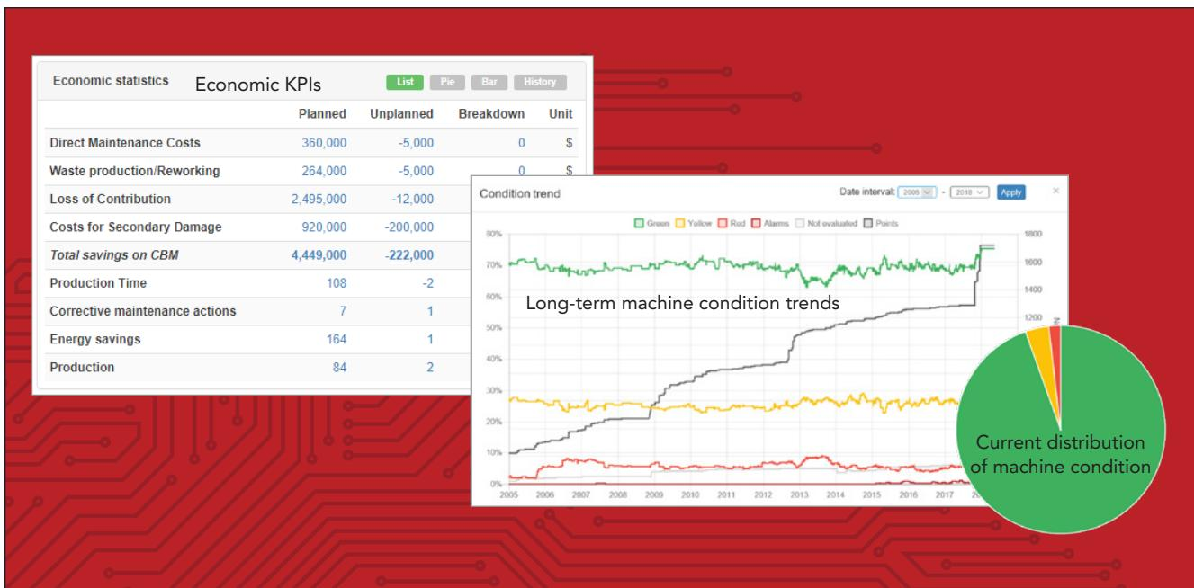
Plant Performer compiles and visualizes statistics relating to technical and economic KPIs (Key Performance Indicators) in the OEE/TEEP area for display and evaluation in Condmaster.NET. Plant Performer, a part of the Condmaster Ruby platform (see TD-583), demonstrates the benefits of condition monitoring and communicates its technical and economic impact to all levels of the organization.
