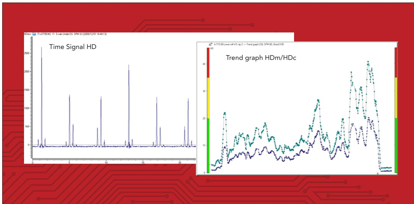
SPM HD Expert is a complement to SPM HDm/HDc and LR/HR. Advanced digital technique, RPM-based sampling frequency and measuring time automatically adjusted to RPM makes SPM HD particularly well suited for measurement on low speed applications. Extraordinary signal quality and 24 bit A/D conversion provides razor-sharp resolution and exceptional detail in spectrums and time signals.
