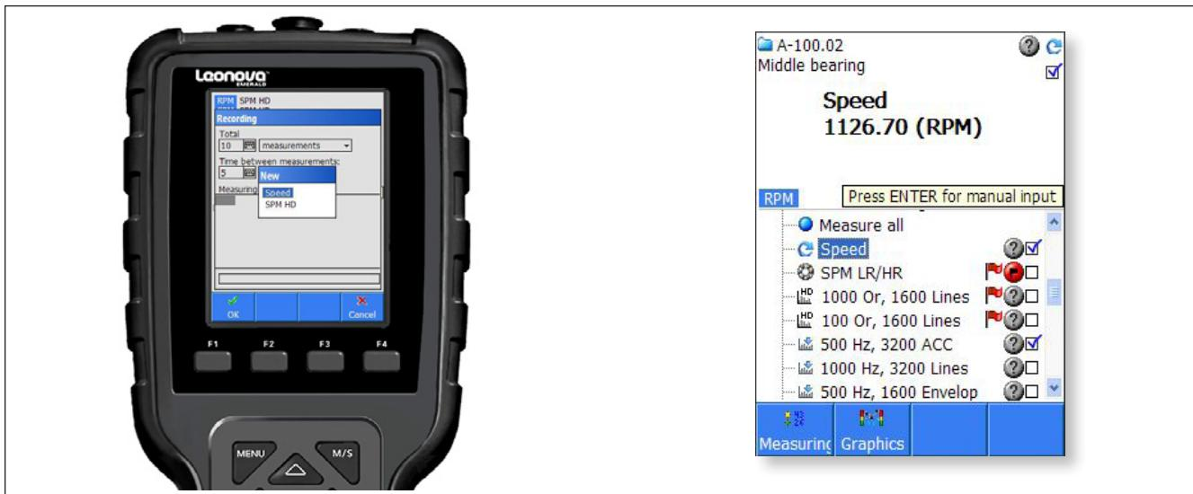
Recording is an Leonova function included in the platform. It allows the user to measure and record measuring results over longer periods of time, up to 50 hours. The recording function is an analysis tool which can show the interaction of various condition parameters over time.
