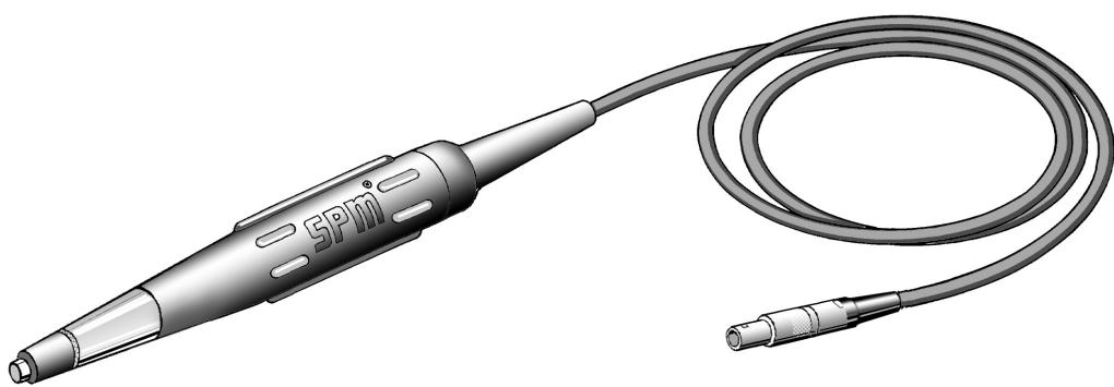
TRA78 is a handheld probe, used together with Leonova Diamond® and Emerald®. The probe is directionally sensitive and must be held aligned against the bearing and not deviate from this direction by more than  $\pm 5^\circ$ . The probe tip is spring loaded and moves within a sleeve made of chloroprene rubber (neoprene) and tolerates 110 °C (230 °F). Standard cable length is 1.5 m. Other lengths up to 20 m can be ordered.
