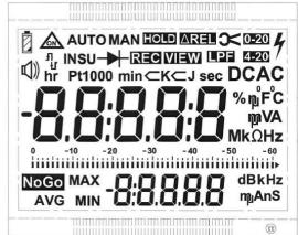
LCD display field 67 mm X 54 mm with digital display, analog scale and with display of measurement unit, and Various special functions.
