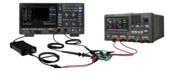
SDS800X HD can control the USB AWG module or control an independent SIGLENT SDG instrument, scan a devices amplitude and phase frequency response, and display the data as a Bode Plot. There is also a Vari-level Mode for accurately measuring Power Supply Control Loop Response (PSRR).
