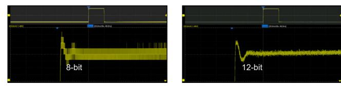
Vertical & Horizontal Zoom along with a large memory depth make the most out of 12-bit ADC resolution. Engineers can observe waveform overall and details simultaneously.
