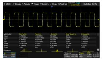
Statistics show the current value, maximum value, minimum value, standard deviation, and mean value. A histogram is available to show the probability distribution of a parameter. Trend and Track are available to show the parameter value vs. time.
