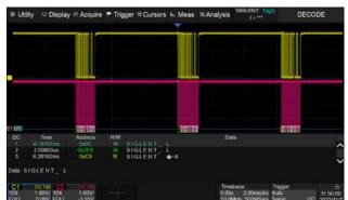
Display the decoded characters through the events list. Bus protocol information can be quickly and intuitively displayed in tabular form. I<sup>2</sup>C, SPI, UART, CAN, LIN are supported.
