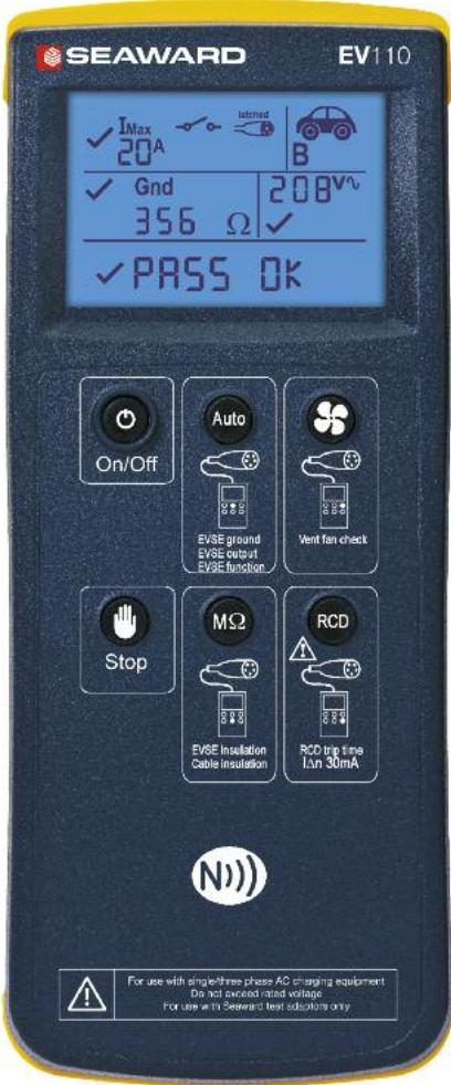
The EV110 is also able to simulate a number of vehicle faults, and automatically store the EVSE fault response including the disconnection time and the amplitude, frequency and duty cycle of the PWM communication between the EVSE and simulated EV.
