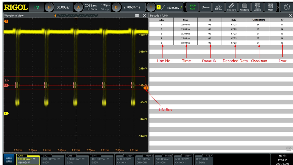
Figure 17.15 LIN Decoding Event Table
