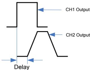
**Note:** The delay function is only for dual-channel models.
