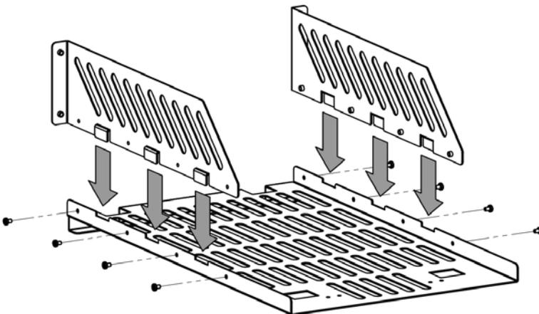
3. Place the instrument: align the protection pads of the instrument with the corresponding holes and then place it on the Support Board.
