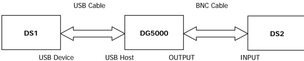
1. Make sure the measured signal is displayed stably on the screen of oscilloscope DS1.
