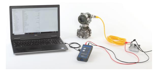
Shown using USB and Foundation Fieldbus (FF)
