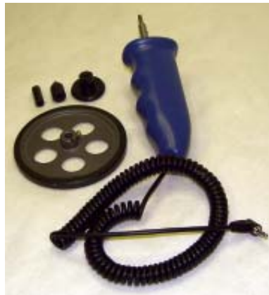
Remote Magnetic Sensor (MT-190-P) Gap 0.25 inches
