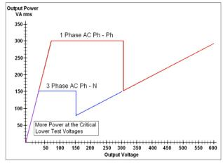
"PowerV" Voltage Amplifier Output Power Curves
