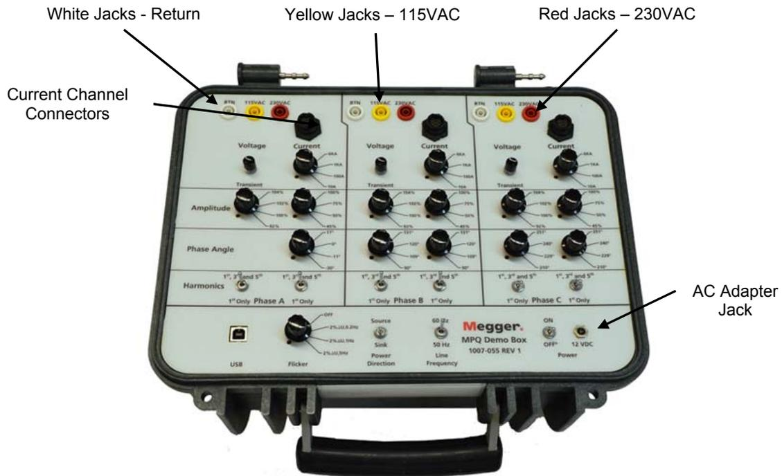
Plug the AC Adapter into the AC Adapter jack of the MPQSIM product.
