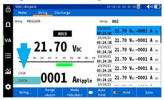
Take measurement of the first cell. The DC voltage and DC current will be saved with a date and time stamp.
