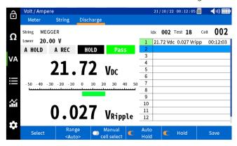
Take measurement of the each following cell. Each measurement shall be saved in sequence with a cell number, date and time stamp.
