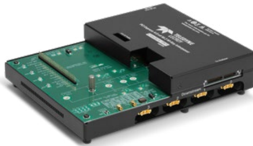
PCI Express 4.0 x4 M.2 M-Key Interposer
