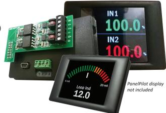
This add-on module interfaces directly with any PanelPilot display from the list below. It provides dual channel 4-20mA galvanic isolation.
