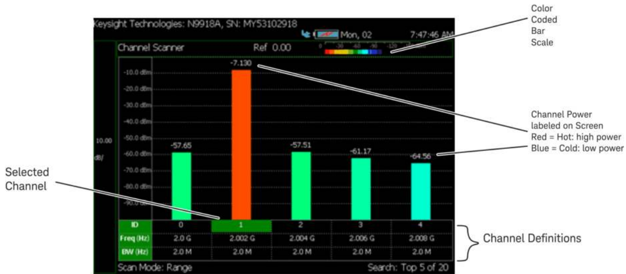
Figure 28-1 Display Example: Measure 5 Channels Spaced 2 MHz Apart
