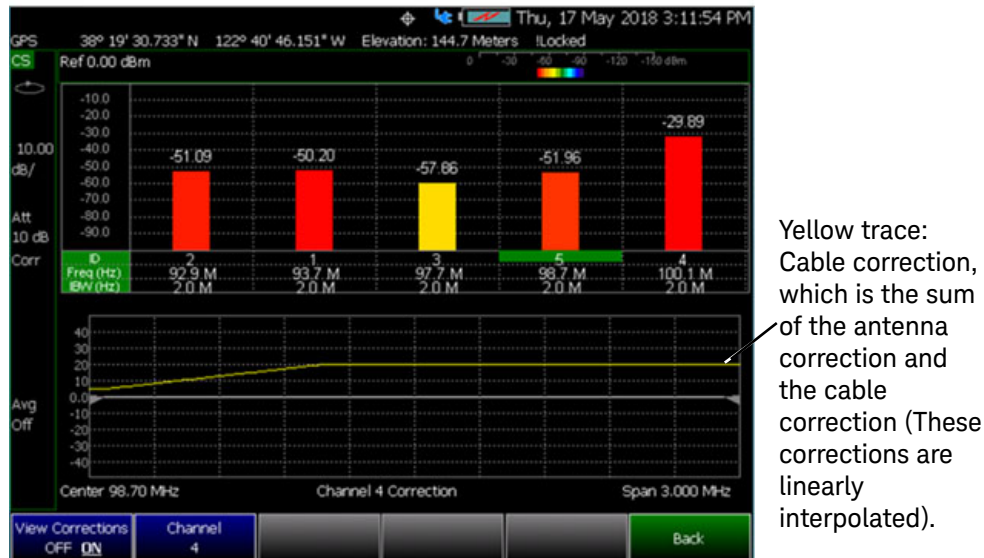
Figure 28-22 Yellow Trace with Cable and Antenna Corrections
