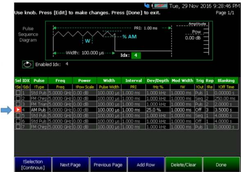
Figure 11 AM triplet with 3.5 s blanking (OFF time) plays continuously with trigger out OFF
