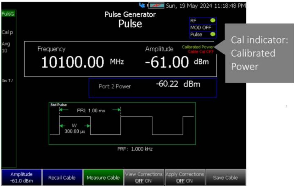
Figure 1 CW = 10.1 GHz is Calibrated and Power Level Below -60 dBm
