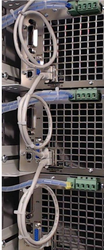
2. Install the **Group** (Master/Slave) cables. These grey CAT5 cables are included in the accessory box shipped with the rack cabinet.
