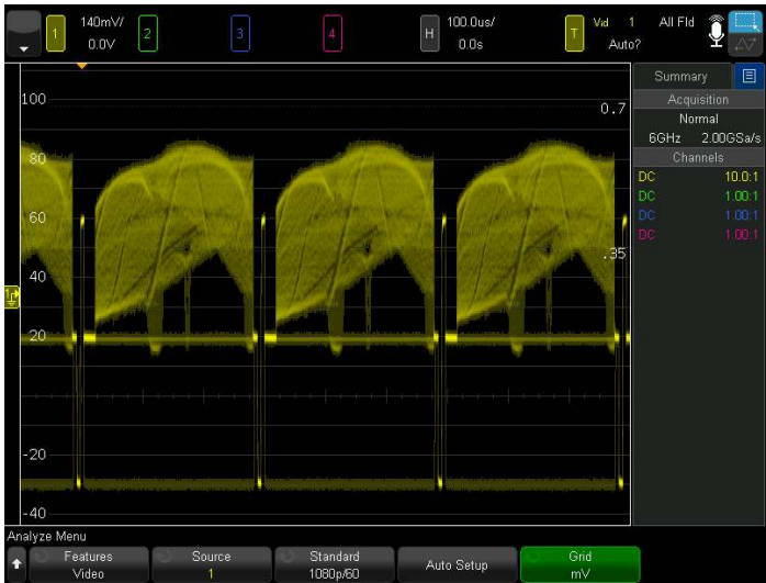
Figure 45. Triggering on a 1080p/60 signal.
