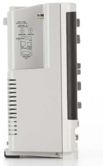
Figure 8. One- gigahertz-per-inch form factor: 6 GHz, 6 inches deep.
