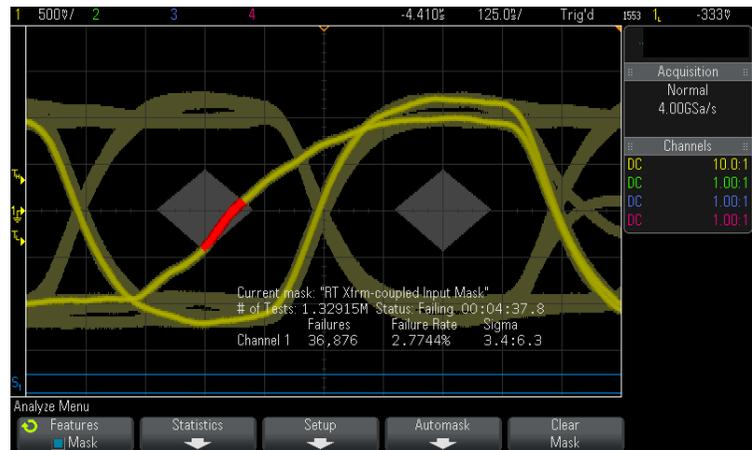
Figure 4. MIL-STD 1553 eye-diagram mask test.
