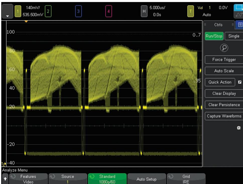
Figure 6. Triggering on 1080p HDTV.
