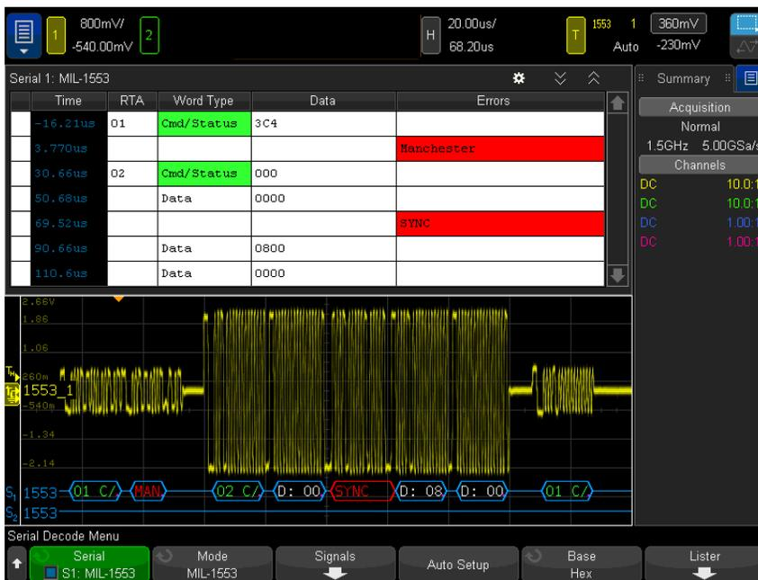
Figure 2. MIL-STD 1553 decode on an InfiniiVision X-Series oscilloscope.
