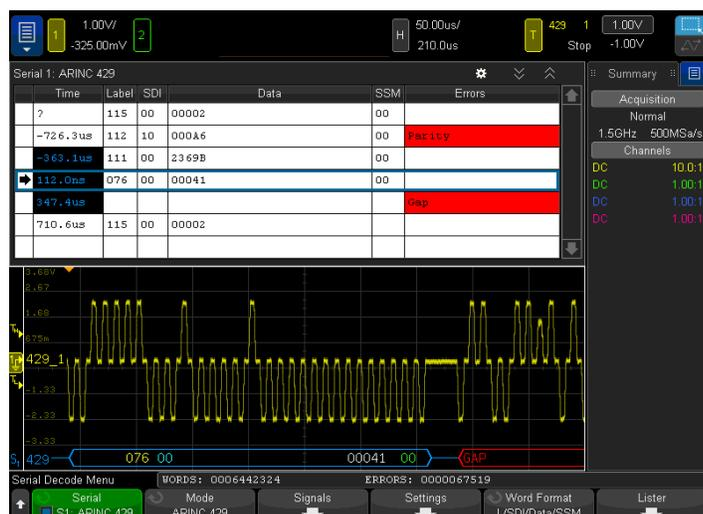
Figure 2. ARINC 429 decode on an InfiniiVision X-Series oscilloscope.
