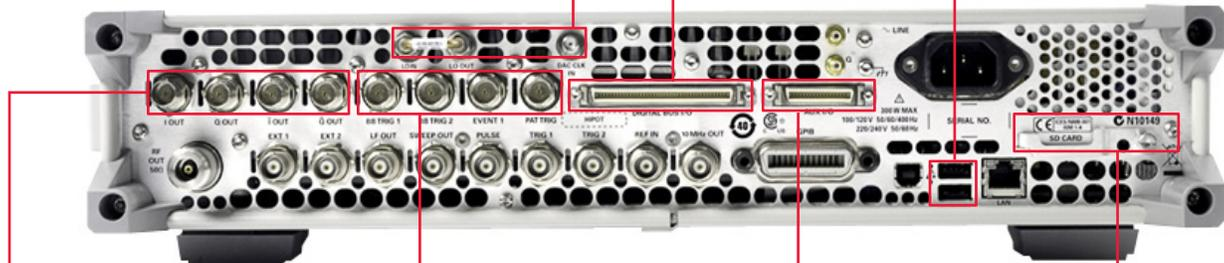
Stimulate baseband I/Q systems with standard single-ended analog I/Q outputs or differential (Option 1EL).
