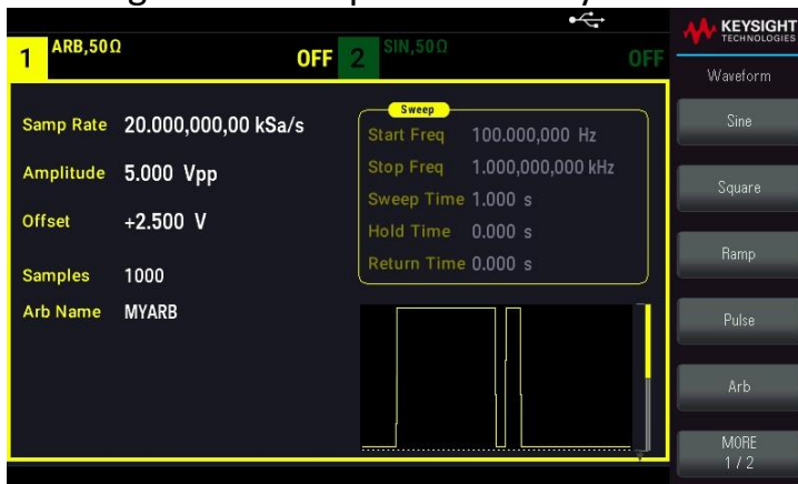
Figure 21 Function Generator with Double Pulse Signal
