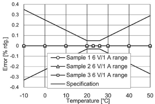
Fig. 17. Active power temperature characteristics: DC (0% f.s.).
