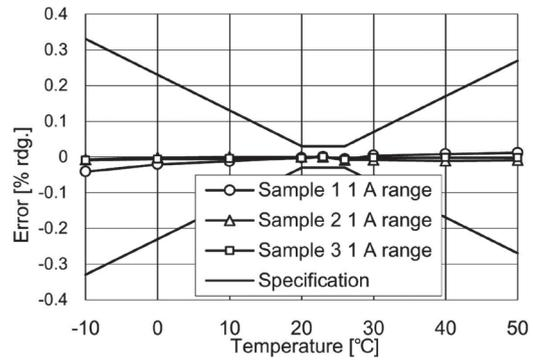
Fig. 15. Current temperature characteristics: DC (0% f.s.).
