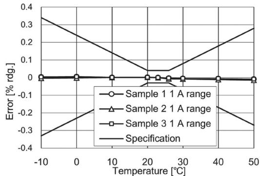
Fig. 16. Current temperature characteristics: AC+DC (100% f.s.).
