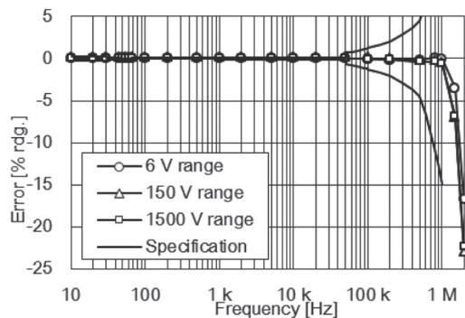
Fig. 9. Voltage frequency characteristics: AC+DC.
