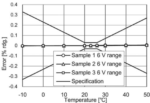
Fig. 13. Voltage temperature characteristics: DC (0% f.s.).
