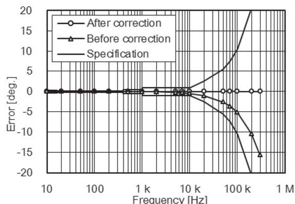
Fig. 2. CT6862 phase characteristics correction.
