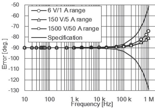
Fig. 12. Phase frequency characteristics: AC+DC.
