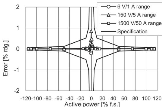
Fig. 7. Active power linearity: DC.
