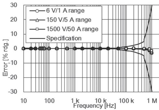
Fig. 11. Active power frequency characteristics: AC+DC.
