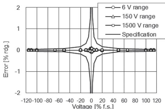
Fig. 3. Voltage linearity: DC.
