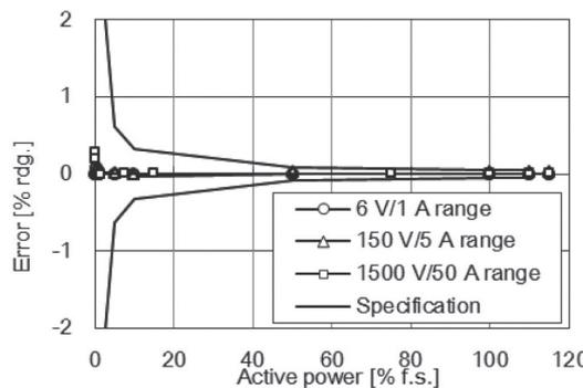
Fig. 8. Active power linearity: AC+DC.
