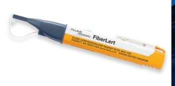
**FiberLert™** lets you quickly check fiber activity, polarity, and connectivity. No setup or interpretation required—just place in front of the fiber end face or port and a light and tone indicate an active fiber. This pocket-sized tool tests single-mode, multimode UPC and APC patch cords and ports using a "non-contact"/ non-contaminating detector.
