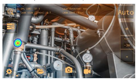
The camera can detect all kinds of pressurized gas leaks and vacuum leaks, by analyzing the sound emitted by the leak. In addition to compressed air leaks, the camera is able to detect leaks of various industrial gases.
