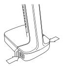
2. Pull the battery out of the camera.
