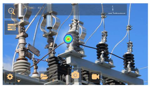
When an electric component begins to fail, one of the first indicators is sound. This sound is caused by partial discharges, that signal the harmful flow of electricity and deteriorate components over time.
