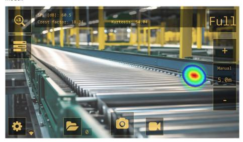
Constant wear and tear of key components in conveyor systems can lead to deterioration. Bearings that are in need of lubrication or are developing faults begin to emit excessive noise.
