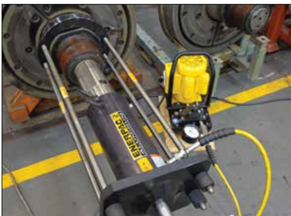
◀ Rail wheel pulling using RACH aluminum cylinder powered by ZE-Series pump.
