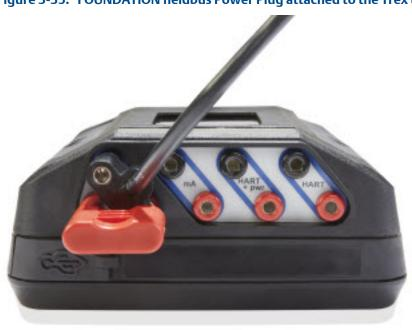
Figure 3-35: FOUNDATION fieldbus Power Plug attached to the Trex unit
