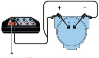
Figure 5-5: Connection for powering a FOUNDATION fieldbus device
