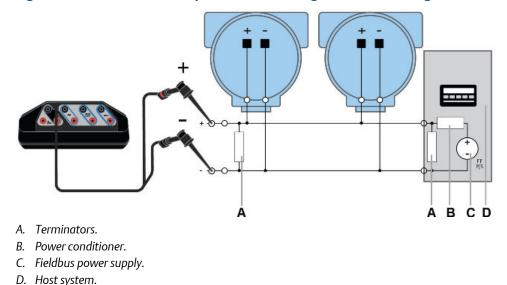
Figure 5-6: One connection option for connecting to the fieldbus segment
