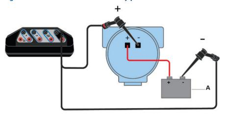
Figure 3-27: Connection for an externally-powered 2-wire transmitter
