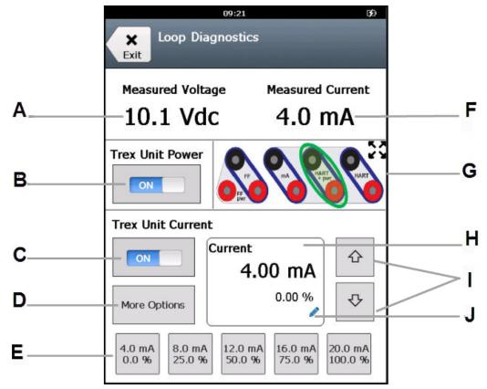
Figure 4-2: Loop Diagnostics when powering a positioner and taking measurements
