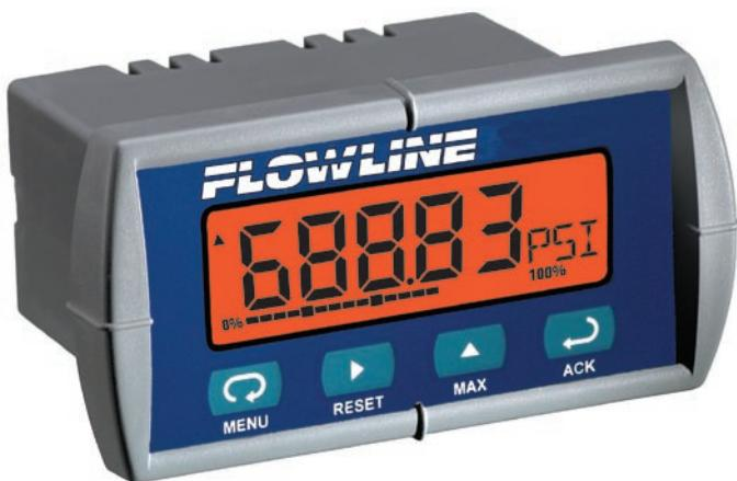
FM and CSA approved intrinsically safe, the loop powered level indicator displays engineering units connected in series with one 4-20 mA continuous level transmitter. Select the LI25-2001 level indicator for hazardous applications with an intrinsically safe sensor. For field mount installation, add a single or two indicator NEMA box.
