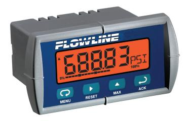
The general purpose loop powered level indicator displays engineering units connected in series with one 4-20 mA continuous level transmitter. For field mount installation, add a single or two indicator NEMA box.
