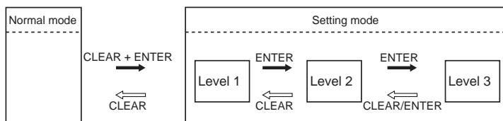
\* You can press the CLEAR + ENTER keys in any level (display) in setting mode to return to normal mode.
