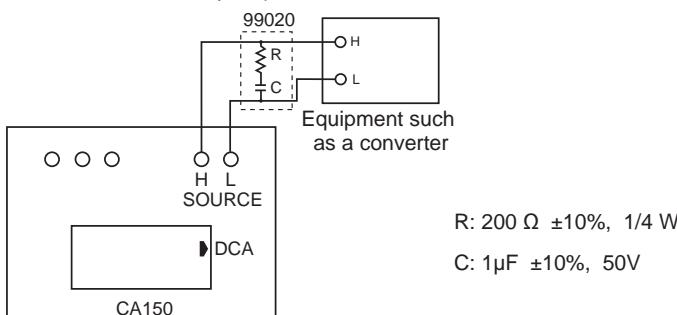
This combination of a resistor (200  $\Omega$ ) and capacitor (1  $\mu$ F) is available as an accessory (Model: 99020).
