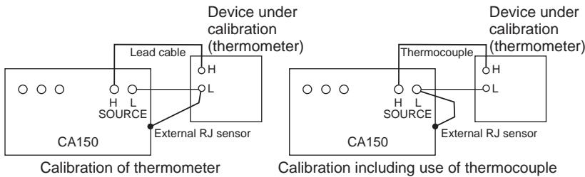
The generation operating procedure is identical to that described in "4.5.1 Generating Thermocouple (TC) Signals."
