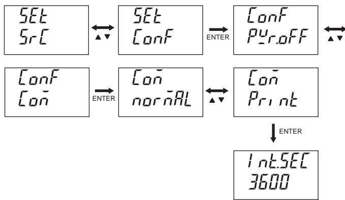
To return to normal mode from setting mode, simultaneously press the CLEAR and ENTER keys.
