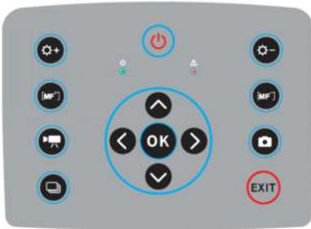
Fig. 16. Arrangement of the control panel buttons.
