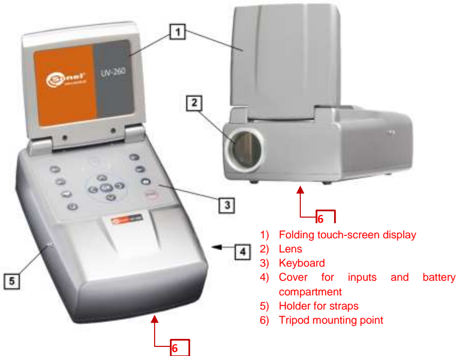
Fig. 11. Parts of Camera UV-260.
