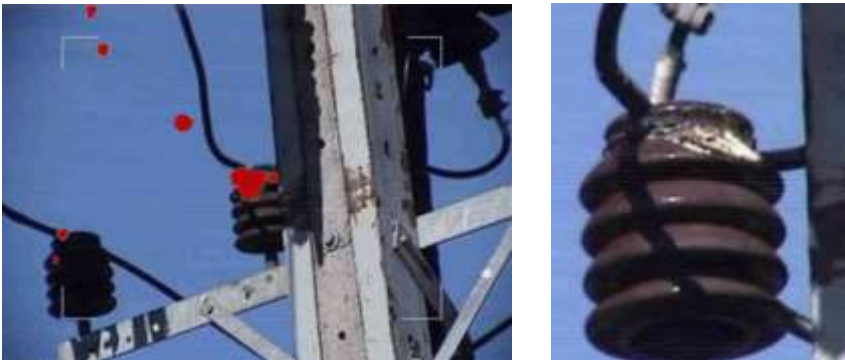
Fig. 9, 10. Corona discharge and its effects.
