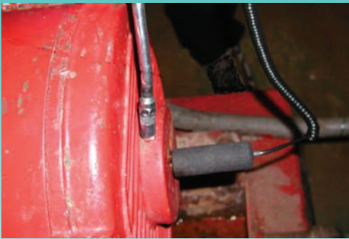
The magnetic mount makes it easy to apply the sensor to most bearing housings.
