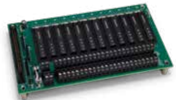
24-channel relay rack PN 52315
