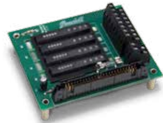
8-channel relay rack PN 52312
