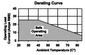
In small enclosures, adequate ventilation must be provided to assure proper safe operating temperature. Accumulation of dust and dirt on the heat sink fins will also affect heat dissipation. In extreme dust and dirt conditions, the relay must be derated by an additional 20%.
