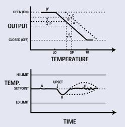
Since the proportional controller is constrained to always operate on its proportional band, the proportional band must be shifted to include the new point "C". A controller with RESET does this automatically.
