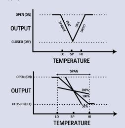
Proportional controllers are tuneable. Their response to process changes can be adjusted to suit the time constants of the specific process system (see figure). In theory, a proportional controller should be all that is needed for process control. Any change in system output is corrected for by an appropriate change in controller output. Unfortunately, the operation of a proportional controller leads to process deviation known as OFFSET or DROOP.
