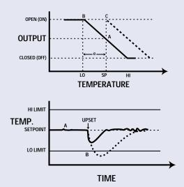
Rate action quickly positions the output where proportional action alone would eventually position the output. In effect, rate action puts the brakes on any offset or error by quickly shifting the proportional band.
