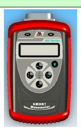
Meriam Process Technologies' M2 Series Products (Smart Manometer and Roots Meter Tester products) are microcontroller based pressure sensing devices used to directly measure pressure. Differential, Gauge, Absolute and Wet/Wet pressure sensors are supported (see Specification section for supported type and pressure ranges). Pressure can be displayed in selectable engineering units of measure.
