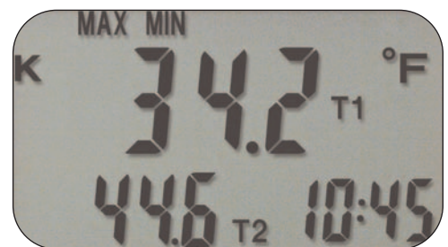
Triple display with backlight shows T1, T2 and relative time stamp.
