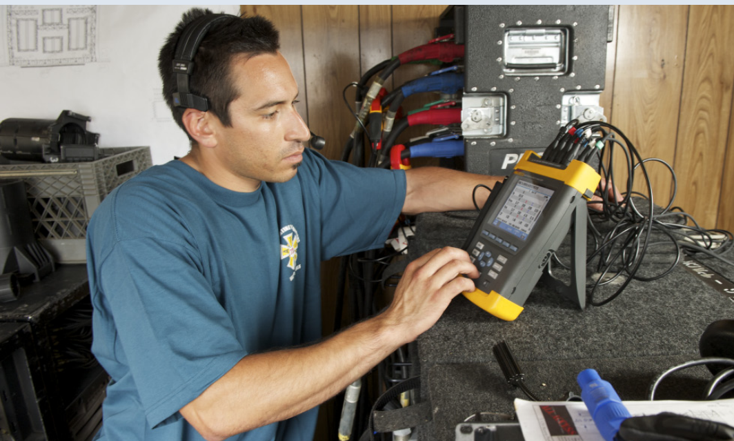
Ruben Esobar, Best Boy Electrician on the set of the Jimmy Kimmel show and a member of Local 728, uses the Fluke 434 Series II Energy Analyzer to look at the individual phases of the power being distributed to the lighting set at an outdoor concert stage. Balancing the power on these systems has been tricky in the past, so he keeps a close eye on them with his 434.
