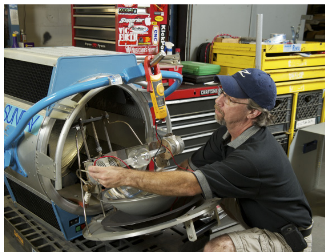
Phil Muskett of DADCO Power and Light checks the continuity of the connection from the ballast to the lamp (lightbulb) holder with a Fluke 337 Clamp Meter. This HMI light fixture is one of the largest light fixtures in the industry at 24,000 kilowatts.
