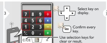
The measurement result from the main line is taken over to the calculator and can be used for further calculations.
