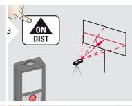
Aim perpendicular to the horizontal center line of the area. This area must be perfectly flat on the vertical plane.
