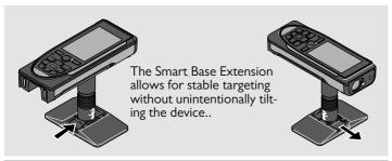
Do not move or tilt the Smartbase during measuring.
