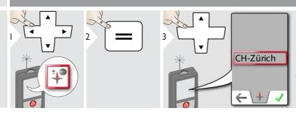
Select the nearest location and the device adjusts the declination accordingly.
