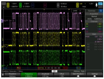
Figure 29. Dual-channel generator generating a differential signal.
