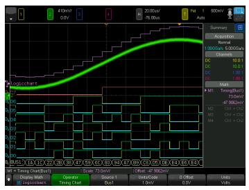
Figure 26. Analog and digital signals displayed together with the logic timing chart function
