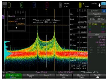
Figure 16a. Color grade and histogram on an FFT function.
