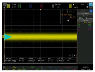
Figure 6. Measuring the noise floor of a 6-GHz scope at 1 mV/div.
