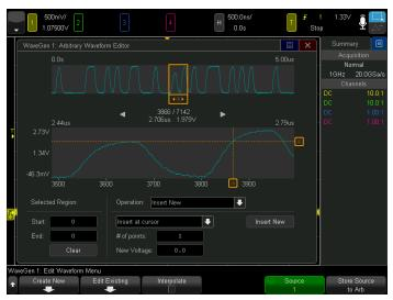
Figure 28. Arbitrary waveform generation signal editing screen.
