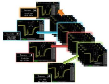
Figure 22. Segmented memory graphical representation.
