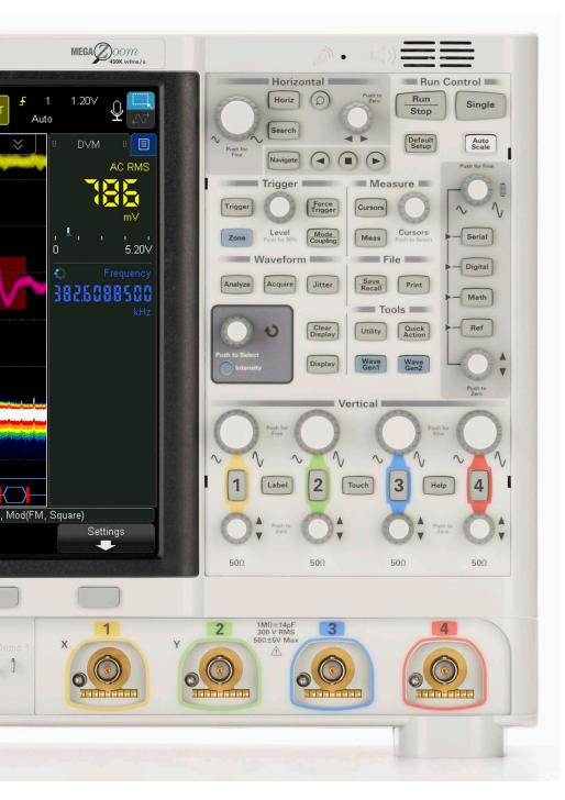
Using docking panels with the capacitive touch screen adds a new dimension of usability. Move automatic measurements, cursors information, event lister, histogram, navigation, DVM, and the counter pane anywhere on the screen. *Transparent* panes are supported.
