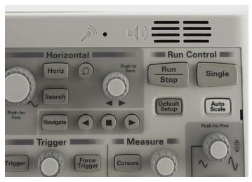
Figure 39. Voice control microphone and speaker.
