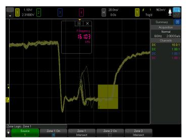
Figure 12. Hardware InfiniiScan Zone triggers immediately.
