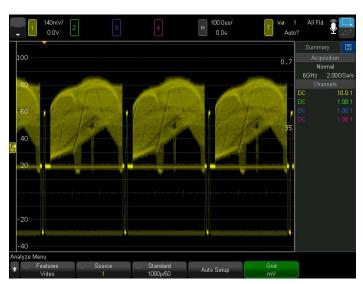
Figure 45. Triggering on a 1080p/60 signal.
