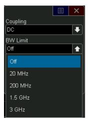
Figure 7. You can set the hardware bandwidth limit control interface per channel at any time.
