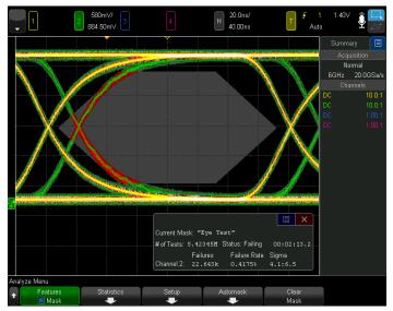
Figure 41. Mask testing of serial data
