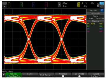
Figure 3. An oscilloscope with 3-GHz bandwidth sees some of the 3rd harmonic of a 2.5-Gbbs PRBS signal.
