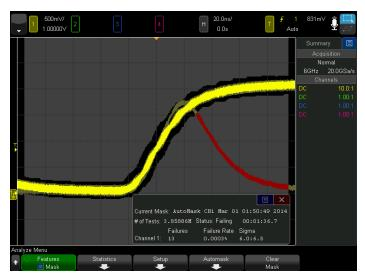
Figure 40. Limit testing of infrequent glitch.
