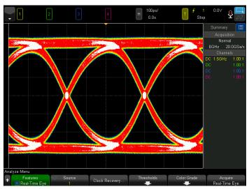
Figure 2. An oscilloscope with 1.5-GHz bandwidth captures only the fundamental frequency of a 2.5-Gbps PRBS signal.
