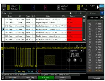
Figure 25. Segmented memory + serial bus decode + InfiniiScan Zone trigger.
