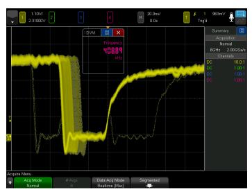
Figure 10. The ultrafast waveform update rate of the 6000 X-Series revealed the existence of rare glitches.
