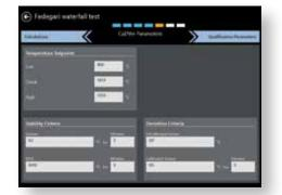
Set the criteria for a sensor calibration - low, high and check point for the actual calibration.
