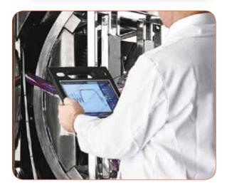
The Kaye Validator AVS system can establish wireless connections\* by utilizing any kind of available Wi-Fi infrastructure like in-house Wi-Fi access points or simply set up a smartphone as a hotspot. This feature simplifies your daily routine work. You can access the live data wirelessly on the console screen while the Validator is wired on the other side of the autoclave. You can start or stop studies and read the live data from a Kaye Validator AVS in a cleanroom without entering the room.
