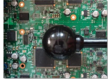
General sphere electric probe, diameter: 3cm
