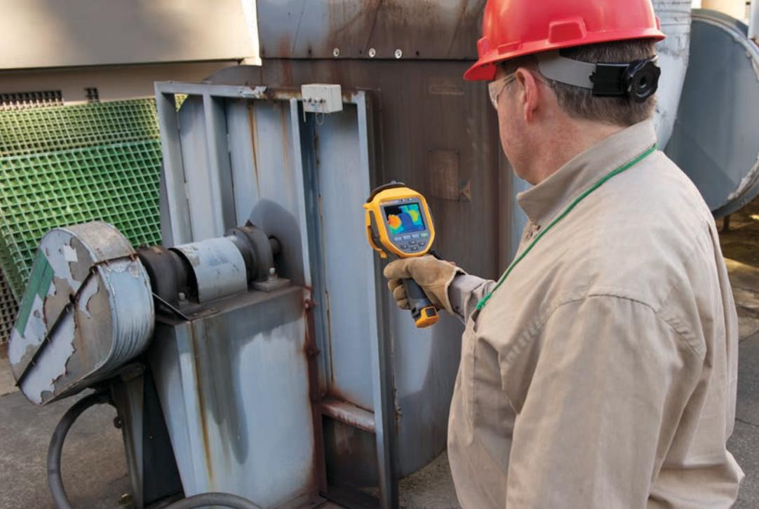
Rising heat becomes visible with a Fluke Ti400 Infrared camera, which captures infrared images of the apparent surface temperatures of all types of equipment.
