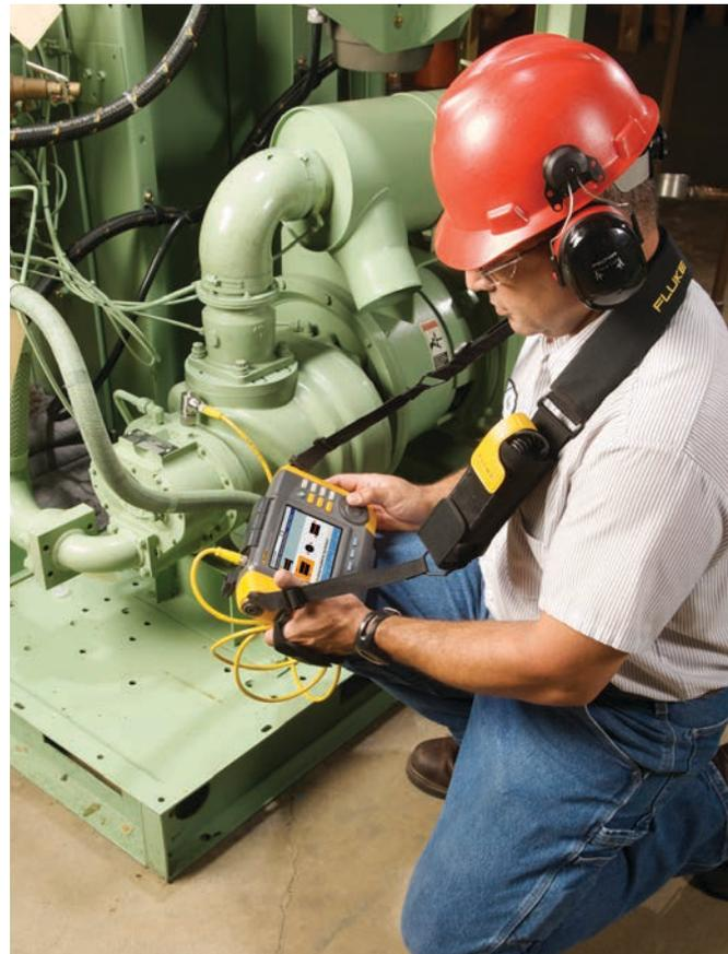
While vibration can be normal in machine operation, it can also be both a sign and a source of trouble. The handheld Fluke 810 Vibration Tester is designed and programmed to diagnose the most common mechanical problems of imbalance, looseness, misalignment, and bearing faults.
