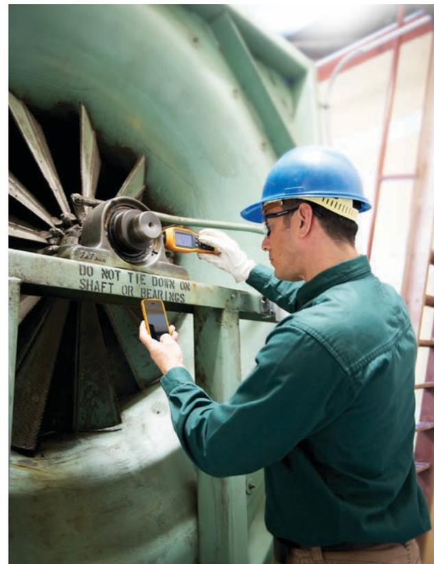
readings over time will help you to know which machines need to be scheduled for repair before a simple bearing failure leads to the loss of the shaft, loss of the machine, or loss of production.
