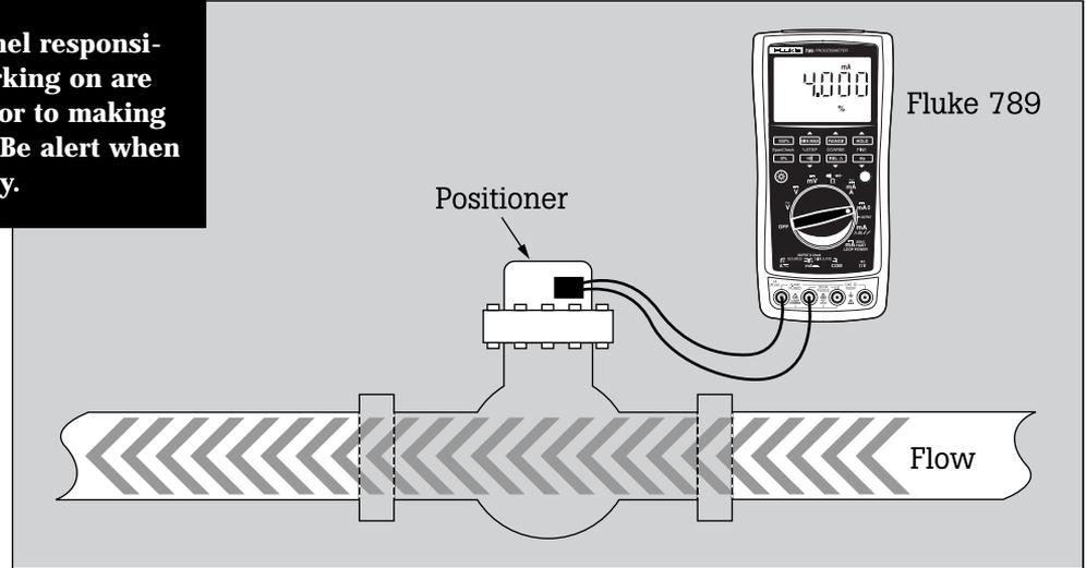
For valves with linear action, linearity can be checked by setting the Fluke 789 to 4 mA and then, using the % Step button, step the current to 12 mA (50 %) and confirm the valve position indicator is at 50 % travel. If your valve is of a non-linear type, refer to the valve manual for proper operation.
